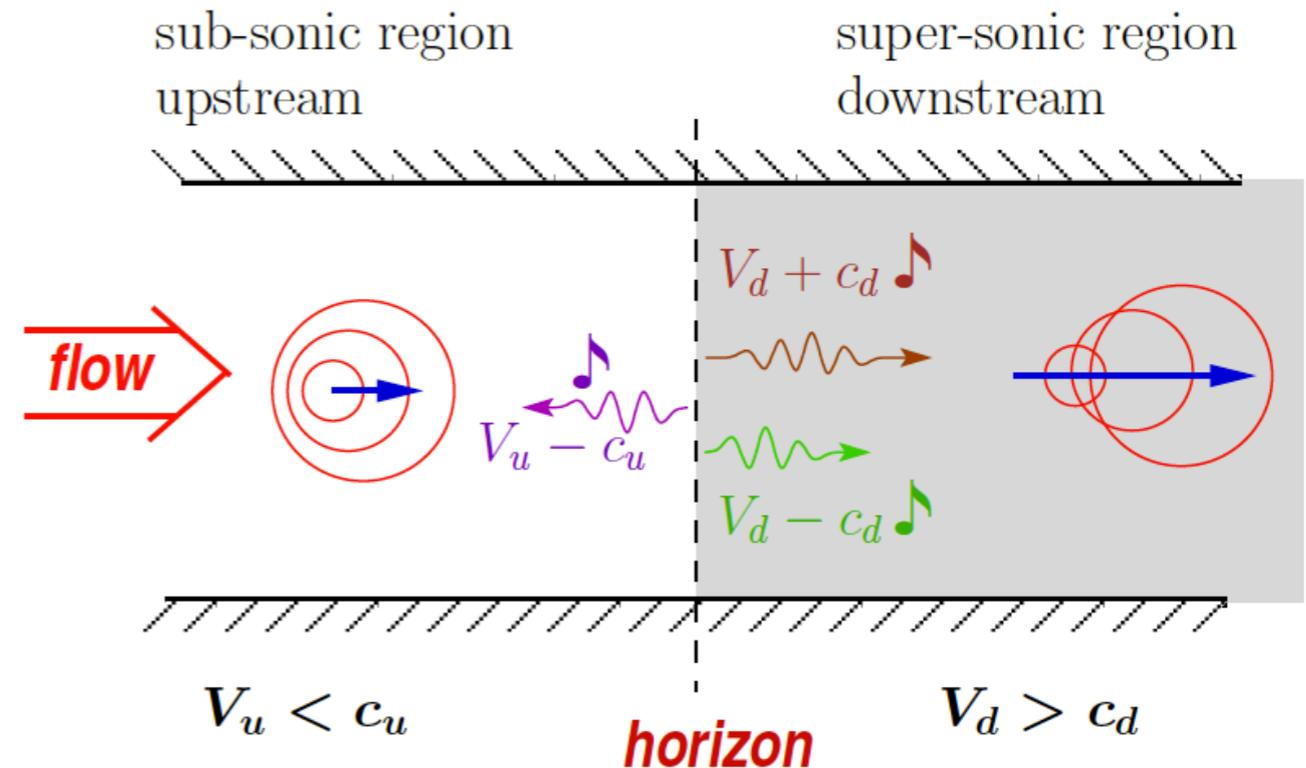
Speed of surface waves relative to flow in a water tank changes. Unruh suggested one could realize a sonic horizon and observe “classical” Hawking radiation Weinfurtner et al. PRL 2011
